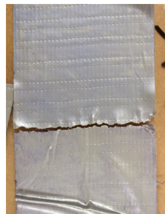
An example of a positive physical fit (Type I Association) between two tape pieces.
